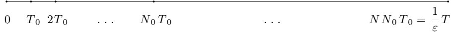
FIGURE 1. Subdivision of the time interval [0, \frac{1}{\varepsilon} T] used in the application of MRCMs. The quality of the approximation is determined by the increment H = \varepsilon N_0 .
